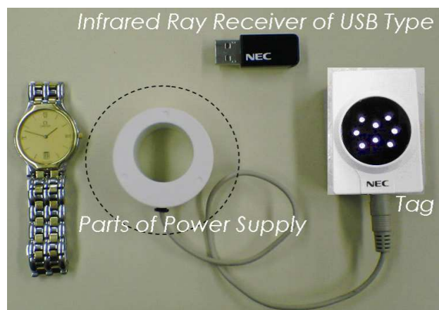
Fig. 4. External appearance of the Lighting Tag and the USB infrared light receiver.
