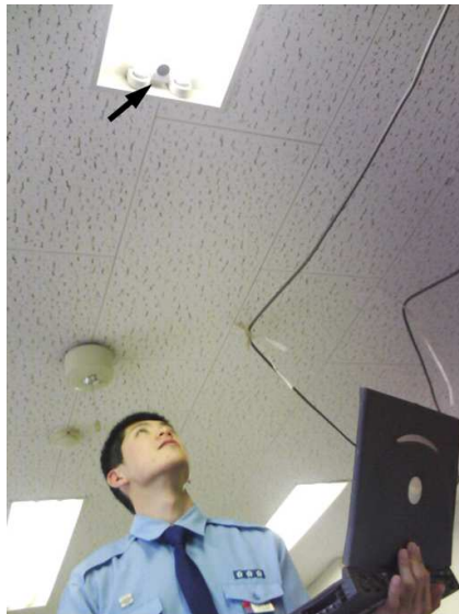
Fig. 5. Experimental ID reception from a Lighting Tag by using infrared light data communication.
