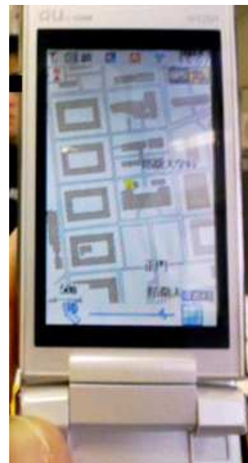
Fig. 1. External appearance of a cellular phone with built-in function for positioning and mapping through the Internet.
