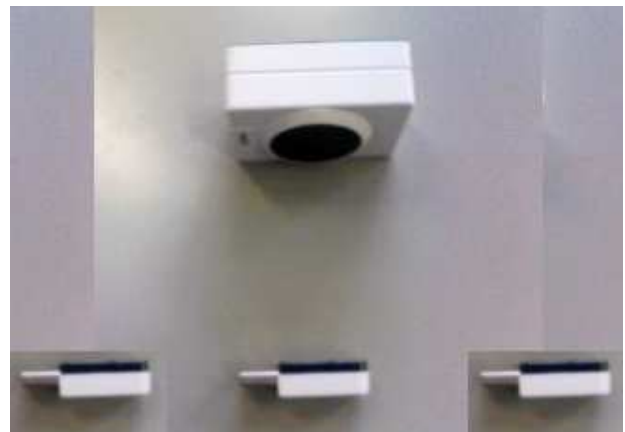
Fig. 7. A conceptual image of ID reception from Lighting Tags by using automatic infrared light data communication, similarly to the case of car navigation.
