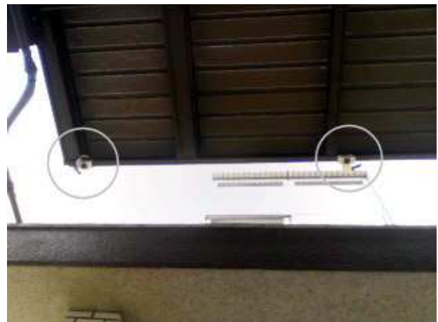
Fig. 13. The exterior appearance of the Lighting Tags installed in the arcade in this mobile experiment.
